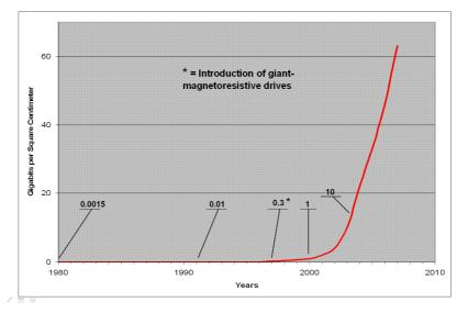
Figure 5. Hard Drive Capacity
