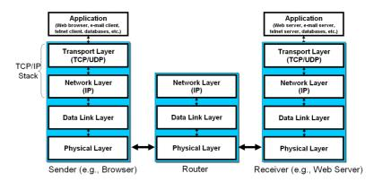
Transmission Control Protocol/Internet Protocol (TCP/IP) stack and the use of a router to transmit packets from the sender to the user.
