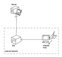
The test was conducted in an artificial environment as represented in Figure 4. The *IDS* in figure is configured as network gateway, so all the traffic coming from the client goes through the *IDS*. It listens to the internal interface sniffing all the traffic. The client using *tcpreplay* replayed the recorded traffic, which was used to train the *IDS* as well as during the execution of the tool.
