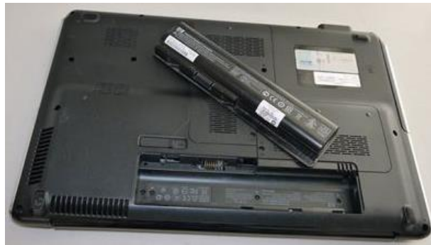
Figure 14. How to remove battery from a laptop (example). 33
