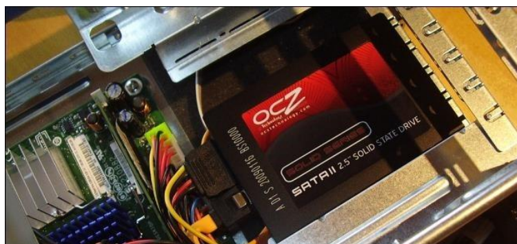
Figure 20. Unplugging the SATA data cable and SATA power cable from the SSD 40 drive [37].
