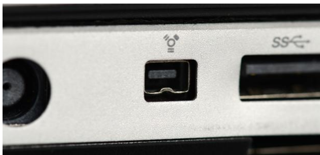
Figure 15. a) Firewire port on the laptop (port in the middle) [29] and b) two Firewire ports [30].
