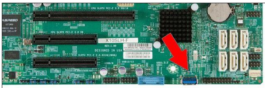
Figure 7. Example USB slot in a motherboard 11 .
