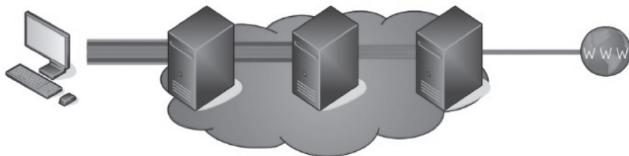
FIGURE 1. FUNCTIONAL PRINCIPLE OF ONION ROUTING. EVERY RELAY ADDS RESPECTIVELY REMOVES ONE LAYER OF ENCRYPTION, AND ONLY KNOWS ITS IMMEDIATE PREDECESSOR AND SUCCESSOR.
