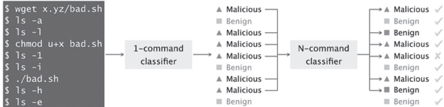
FIGURE 8. THE 1-COMMAND CLASSIFIER IS USED AS A FILTER AND ONLY COMMANDS CLASSIFIED AS MALICIOUS BY THE 1-COMMAND CLASSIFIER ARE PROVIDED TO THE 4-COMMAND CLASSIFIER. THUS, THE 4-COMMAND CLASSIFIER IS PRESENTED WITH A SEQUENCE OF COMMANDS THAT IS AN APPROXIMATION OF THE ORIGINAL MALICIOUS SEQUENCE.
