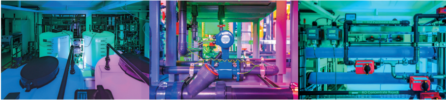
FIGURE 4: (FROM LEFT TO RIGHT) WATER TANKS AT THREE DIFFERENT STAGES OF THE SWAT TESTBED, A FLOW METER SENSOR, AND AN ACTUATOR IN THE FORM OF A MOTORIZED VALVE
